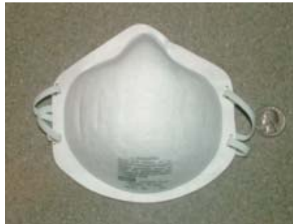
Fig 5. Industrial mask prevented colonization on agar plates, demonstrating protection from aerosolized bacteria.
