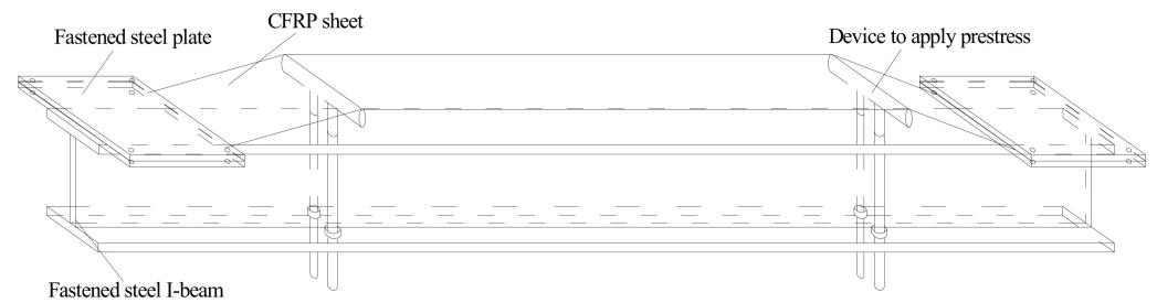
Figure 2. Device for applying prestress to CFRP sheet.
