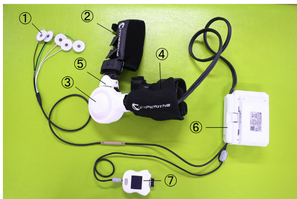
Figure 1. Product components of HAL-single-joint for elbow motion. ①, Electrodes; ②, Upper arm attachment; ③, Ring LED; ④, Forearm attachment; ⑤, Power unit; ⑥, Control box storage bag; ⑦, Controller.
