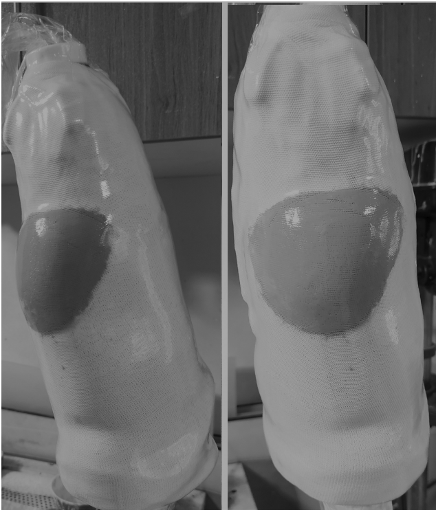
FIGURE 2 Silicone was applied for each layer of fabric on the antero-distal part of tibia. Five layers of fabric were placed on the first layer. The silicone pouring method was same as the first layer. This pouring method was applied for each layer of fabric.
