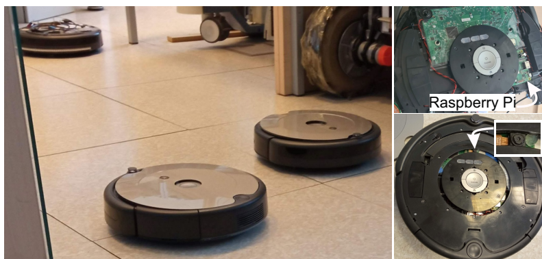
Figure 14. Roomba robots used to simulate transportation tasks in the laboratory layout from Figures 15 and 16. View of the robots (left) and closer robot view with integrated Raspberry Pi and camera (right).
