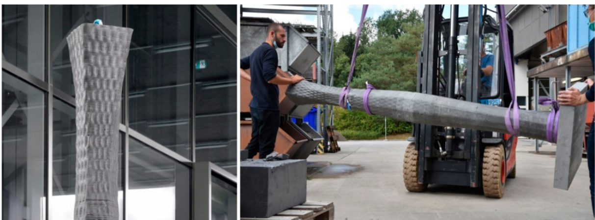
Figure 13. (Left) zoom of cast eggshell columns after demolding; (right) transport of column.
