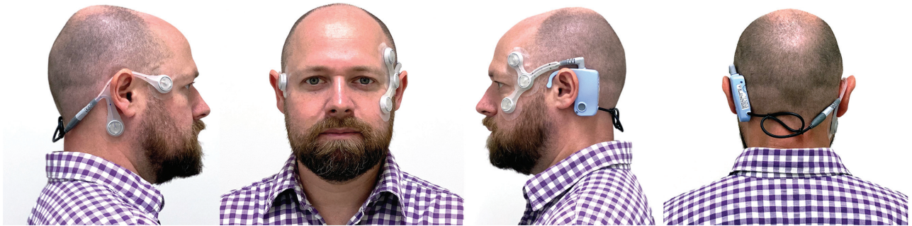
Figure 1. The CAVA (Continuous Ambulatory Vestibular Assessment) device. Two electrodes either side of the eyes record horizontal eye movement, two above and below one eye record vertical eye movement, and a fifth beneath the right ear provides a reference voltage.
