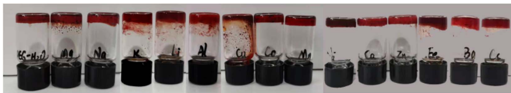
Fig. 7 Cation-responsive of compound 1 when stimulated with metal cations. From left to right, the cation is Na + , Mg 2+ , Na + , K + , Li + , Al 3+ , Cu 2+ , Co 2+ , Mn 2+ , Ni 2+ , Ca 2+ , Zn 2+ , Fe 3+ , Ba 2+ , and Cs + , respectively.
