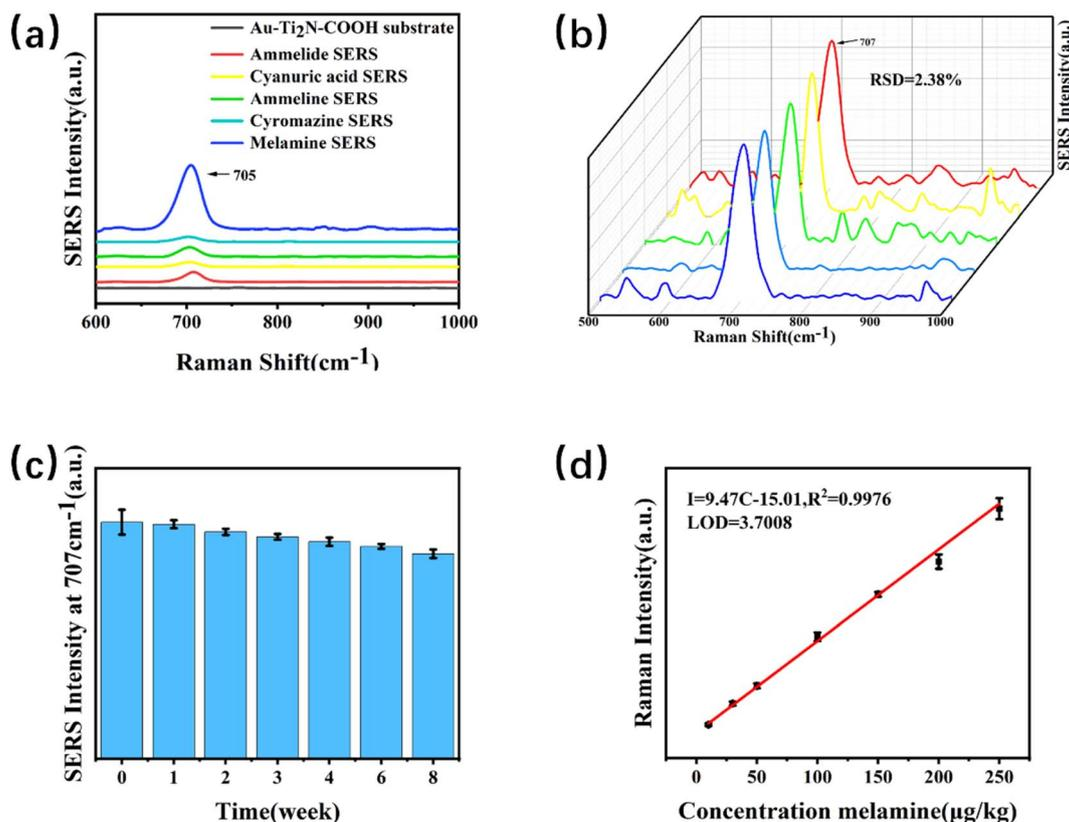
Fig. 5 (a) SERS characteristic peaks of different target substances. (b) SERS spectra of melamine (100 μg kg<sup>-1</sup>) were measured from 5 samples. (c) SERS characteristic peaks of melamine at other time points. (d) Calibration curve of melamine in milk.
