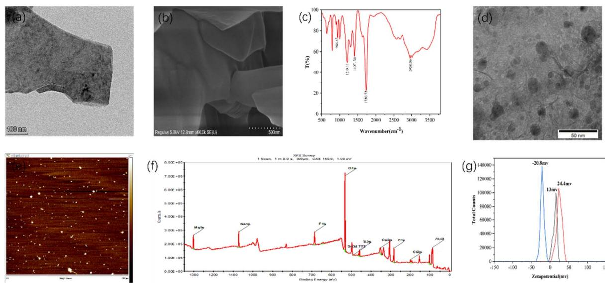
Fig. 2 (a) TEM image of  $\text{Ti}_2\text{N}$ . (b) SEM image of  $\text{Ti}_2\text{N}$ . (c) Infrared spectroscopy of  $\text{Ti}_2\text{N}-\text{COOH}$ . (d) TEM image of Au- $\text{Ti}_2\text{N}-\text{COOH}$ . (e) AFM of Au- $\text{Ti}_2\text{N}-\text{COOH}$ . (f) XPS survey spectrum of Au- $\text{Ti}_2\text{N}-\text{COOH}$ . (g) Zeta-potential of  $\text{Ti}_2\text{N}$ ,  $\text{Ti}_2\text{N}-\text{COOH}$  and Au- $\text{Ti}_2\text{N}-\text{COOH}$ .
