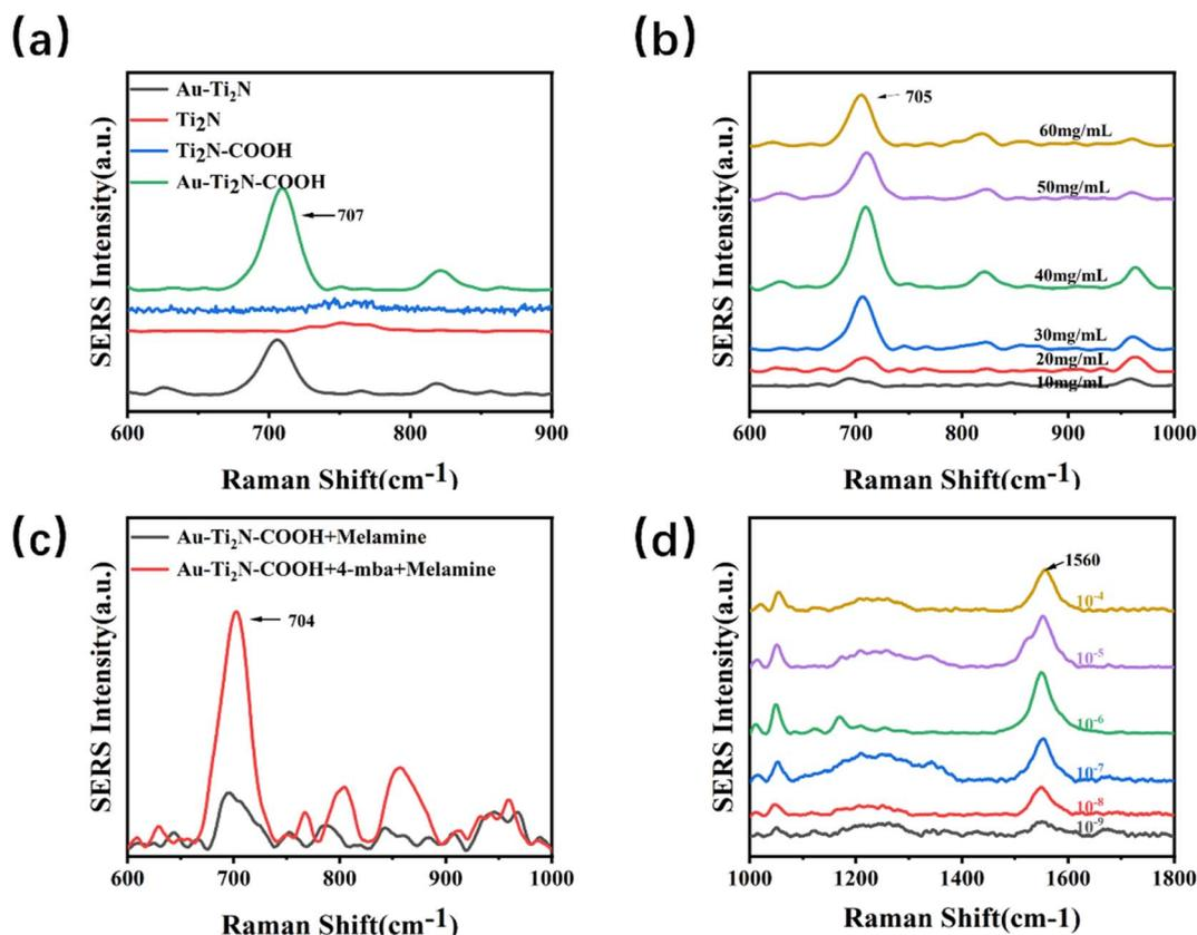
Fig. 4 (a) SERS characteristic peaks at  $707\text{ cm}^{-1}$  for four different substrates (b) the SERS characteristic peak at  $707\text{ cm}^{-1}$  in substrate detection exhibits different intensities at various concentrations. (c) The relationship between Raman intensity and 4-MBA. (d) The relationship between different concentrations of 4-MBA and SERS characteristic peak values.
