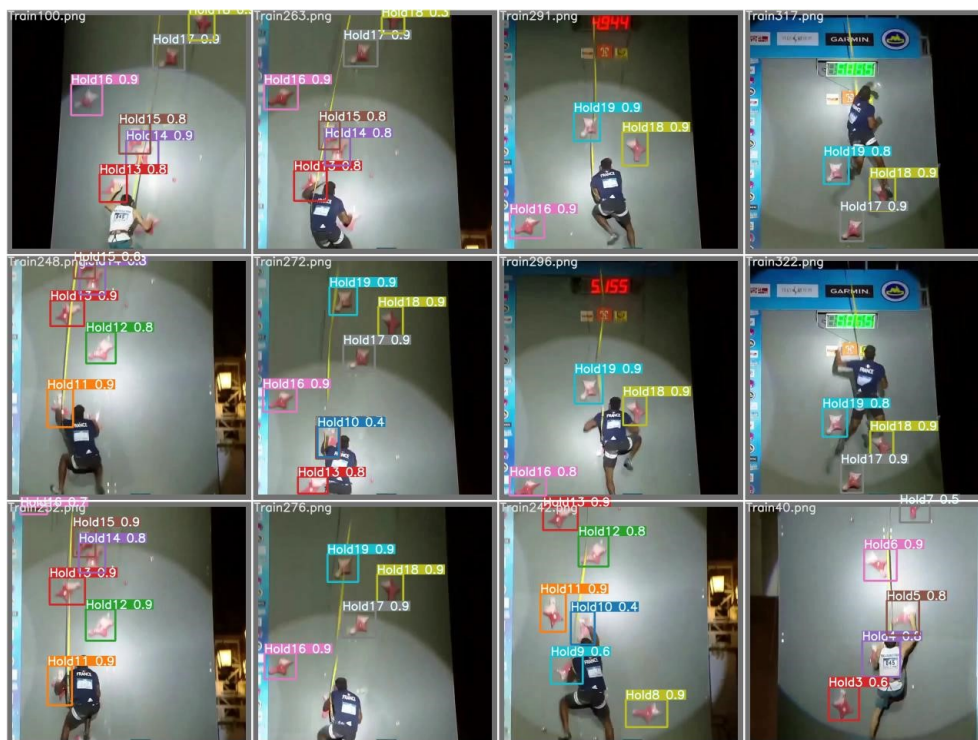
Figure 6. Resulting test batch of a set of images for the detection of speed climbing holds [17].
