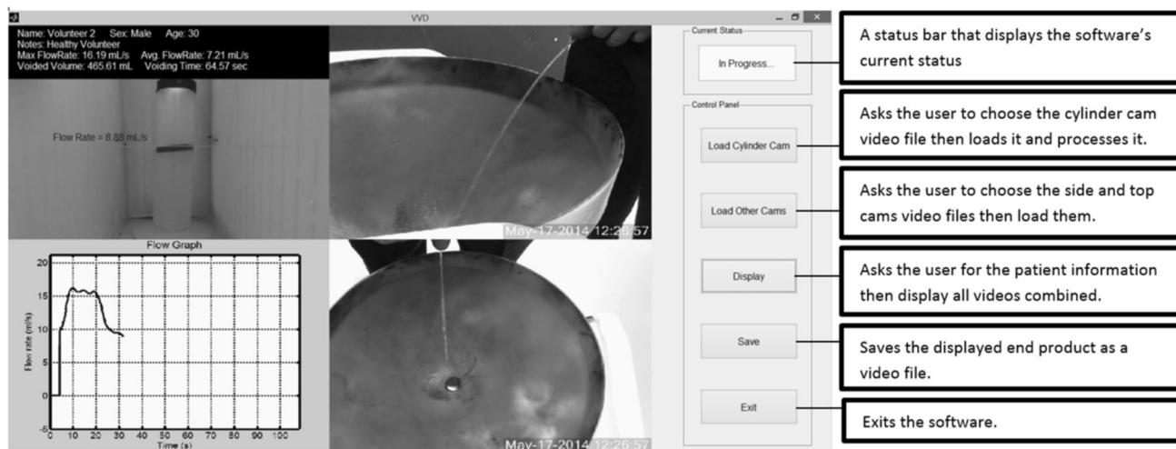
Fig. 7 Screenshot of the VVD software mid-voiding displays all three cameras, patient information, uroflowmetry results, and a live flow graph
