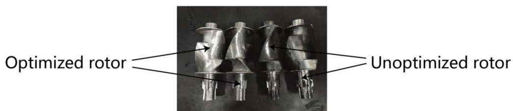
Figure 7. Comparison of internal mixer rotor expansion before and after optimization (photograph of specimens).
