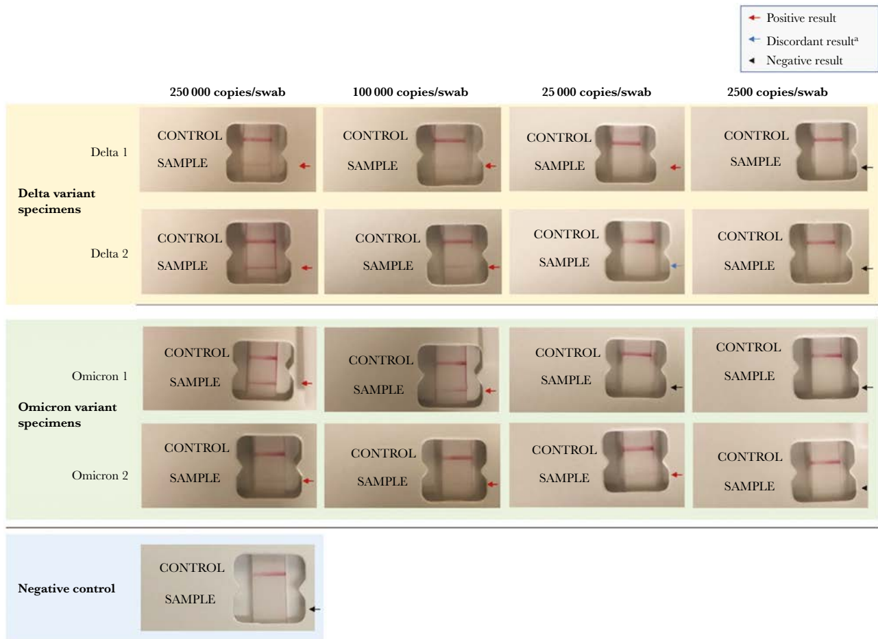
Figure 1. Results of a laboratory-based analytic validation of the BinaxNow SARS-CoV-2 rapid antigen assay across a range of concentrations with both Delta and Omicron variant viruses. For the discordant result, 2 reviewers reported a negative result and 1 reported a positive result. a Discordant results indicate those in which there was not agreement between the 3 blinded readers of each test. Abbreviation: SARS-CoV-2, severe acute respiratory syndrome coronavirus 2.
