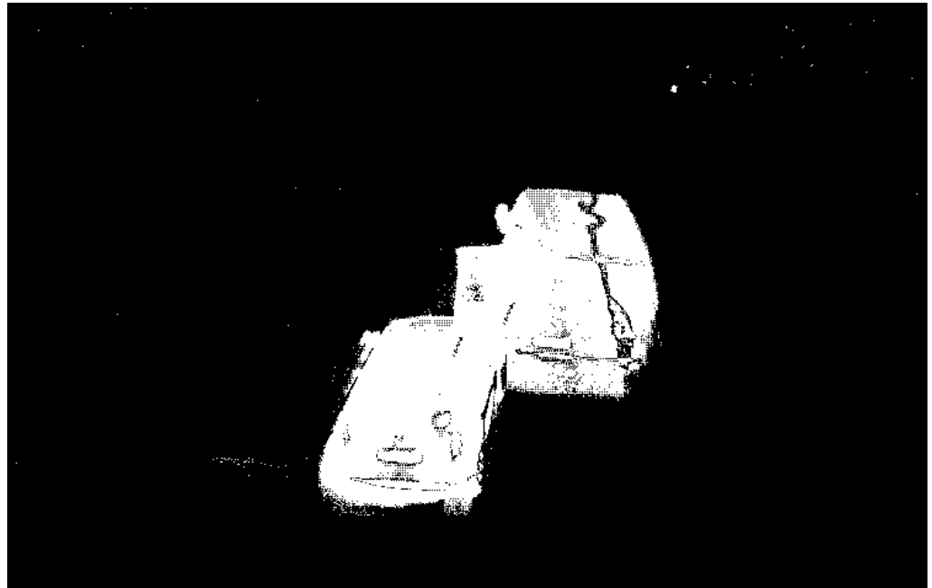
Figure 1. Illustration of a binary mask, obtained by GMM, which contains overlapped vehicles.
