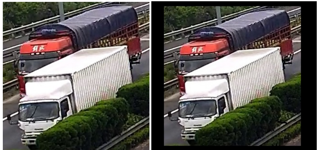
Figure 5. The shape-normalization consists of adding black pixels to an image ( left ) to obtain a new image ( right ) with the desired shape.
