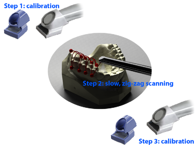
Figure 4. The hi-res scanning protocol for the Lava COS scans. The scanning protocol for the scans for the Lava COS is the normal scanning protocol, except that the scan-path is a slow zigzag scan and that at the end of the scan a second calibration is performed. doi:10.1371/journal.pone.0043312.g004
