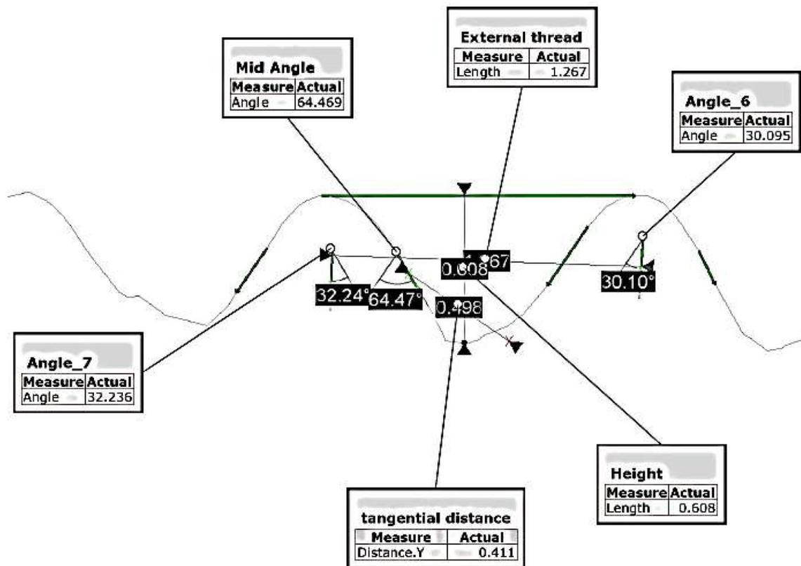
**Fig. 3** Analysis of the geometric features of M8 mild steel's thread profile
