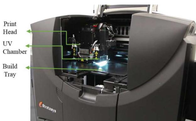
**Fig. 5** Stratays Object 260 Connex 3 polyjet 3D printer
