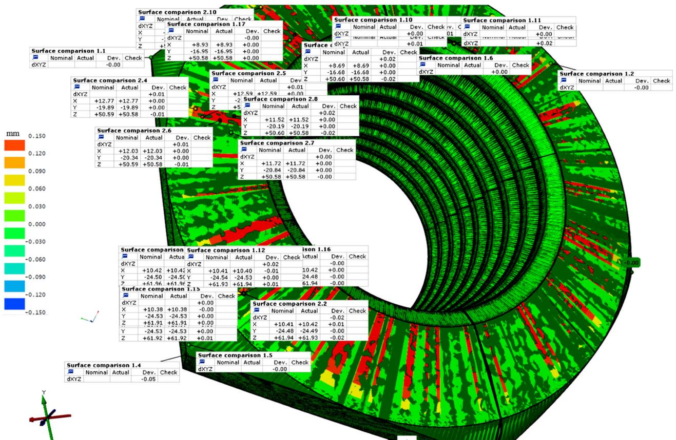
**Fig. 11** Dimensional deviation illustration for Vero thermoplastic AM nut using gray-colored resin
