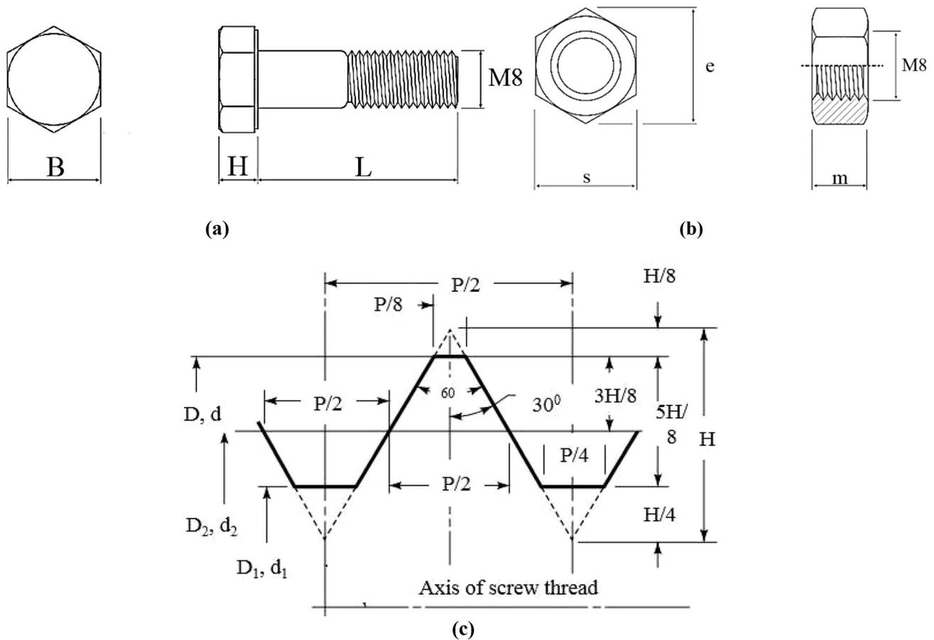
**Fig. 2** a M8 bolt's dimensions. b M8 nut's dimension. c Thread geometry according to ISO 68-1
