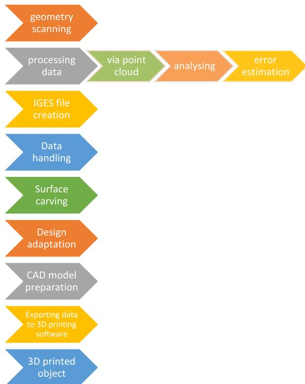
**Fig. 1** Three-dimensional scanning and inspection for reverse manufacturing
