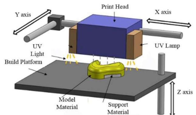
**Fig. 4** Schematic of polyjet printer
