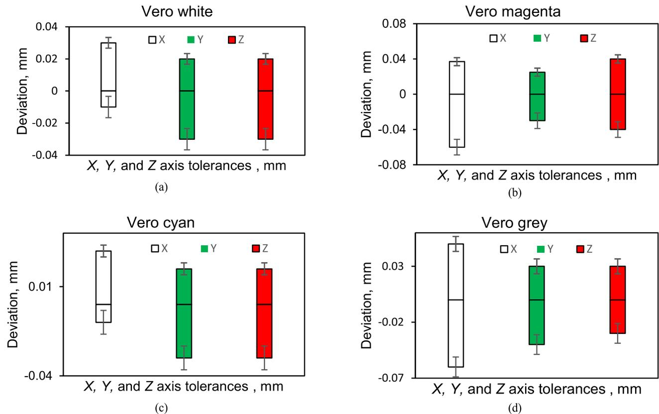
**Fig. 12** Mean dimensional tolerances for the M8 fasteners fabricated using **a** Vero white, **b** Vero magenta, **c** Vero cyan, **d** Vero gray thermoplastics
