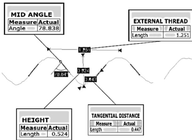
**Fig. 8** Analysis of the geometric features of Vero cyan's thread profile
