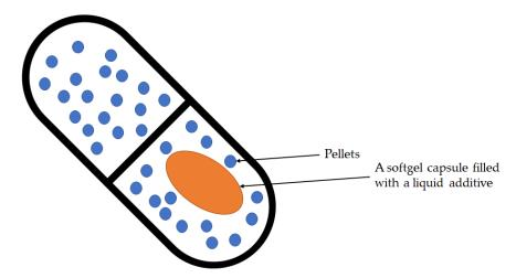
**Figure 1.** The structure of the Combodart/Jalyn: A softgel capsule filled with a liquid additive. The above softgel capsule was introduced into a hard size-00 HPMC capsule. Pellets from the other additive fill the HPMC capsule to accompany the softgel in the final dosage form.
