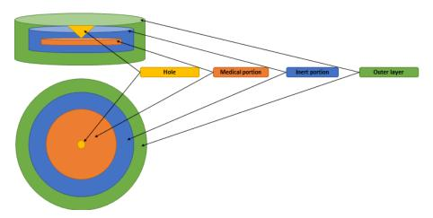
Figure 4. Bilayer tablet according to the Stephenson patent from 1964 [23].
