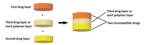
Figure 5. Diagram of a multilayer tablet structure.
