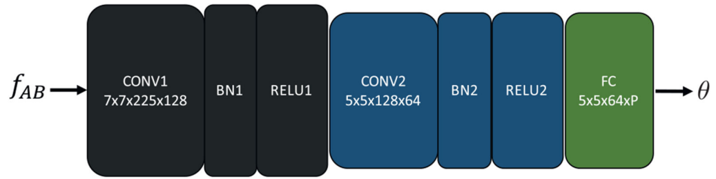
Fig. 3. Regression network for estimating transformation parameters from the correspondence map f_{AB} Rocco et al. (2017).
