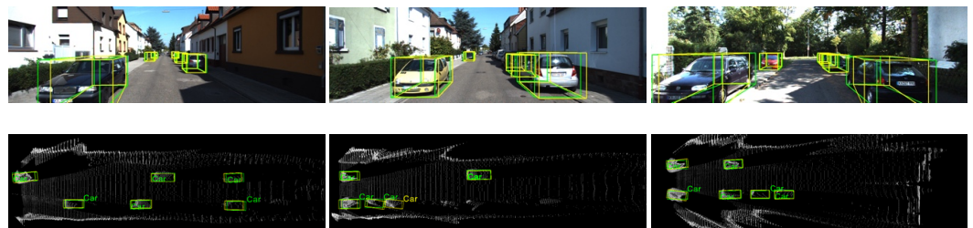
Figure 8. Detection of cars at different distances with occlusion. Top row images are frontal-view images, and bottom row images are bird’s-eye-view point cloud maps. Ground truth boxes are in green and prediction results are in yellow. Our proposed framework is able to create accurate 3D boxes at different distances and for occluded targets.
