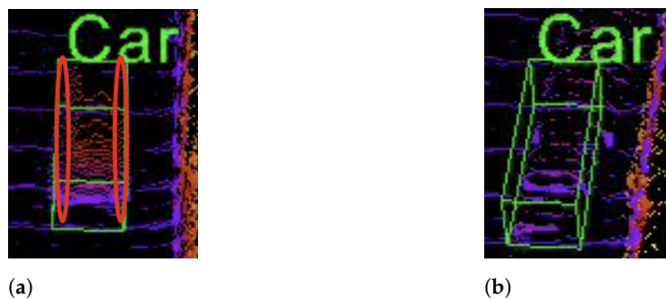
Figure 4. Comparison of 3D detection using: (a) a 2D bounding box; (b) 2D instance segmentation. Ellipses in Figure 4a denote the noise point clouds lying between the boundary and the bounding box of a certain object.
