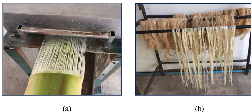
Fig. 4. Banana pseudostem (a) banana pseudostem extraction, (b) dried banana fiber.
