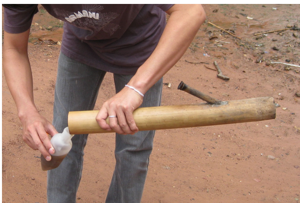
Figure 2. A field laboratory technician pouring water from the TWP into a sample collection bottle.
