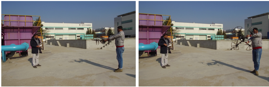
Figure 6. UAV calibration at the experimental site: (Left) Holding it horizontally and (Right) vertically.
