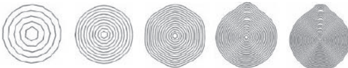
Figure 8. Cross-sectional views of relaxed MWNTs indexed by (2,8)/(4,16)/\dots/(2n,8n) . The wall numbers n are 5, 10, 15, 20, and 25 from left to right, and all the MWNTs are 20 nm long. Reprinted from Reference [63].
