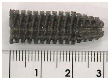
Figure 7. ACL screw from PLA-Mg-vitamin E (Composition 1).
