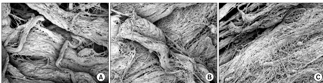
Fig. 6. Electron microscopic findings (after the fatigue test). (A) Glutaraldehyde fixation only; (B) glutaraldehyde fixation+decellularization; (C) glutaraldehyde fixation+decellularization+ \alpha -galactosidase. Interstitial derrangement was observed in B and C. C had more deranged interstium than B ( \times 3,000 ).
