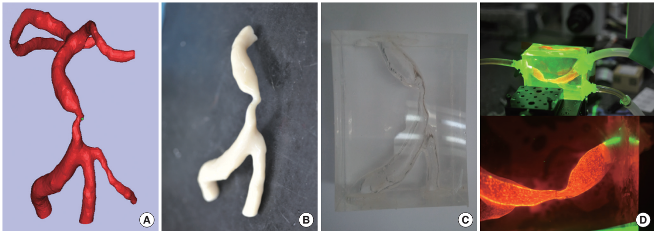
Figure 2. 3D-printed vascular stenosis model and particle image velocimetry (PIV). (A) 3D-reconstructed basilar artery (BA), (B) 3D-printed fabricated model, (C) the silicon cast, and (D) blood flow measurements using PIV.
