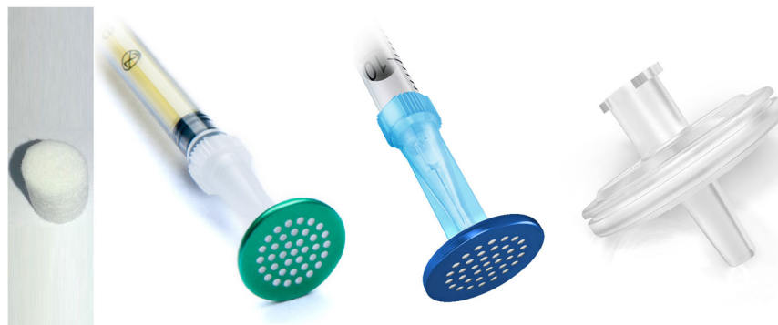
Fig. 1 Filters used. From the left to the right: cotton filter, Sterifilt, Sterifilt +, Minisart “wheel filter”
