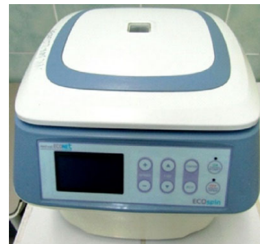
Figure 7 – Centrifuge with sealed rotor or safety cups (authors' collection).
