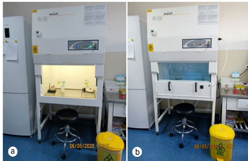
Figure 6 – (a and b) Certified biosafety cabinet (BSC) during working and during its disinfection with ultraviolet C (UVC) light (authors' collection).
