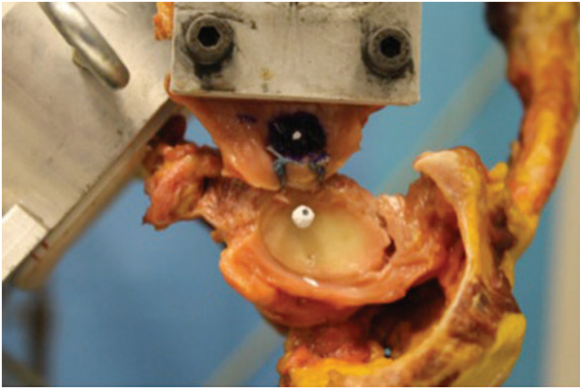
Figure 4. The specimen loaded onto the materials testing apparatus. Tracking markers are placed on the glenoid and capsule for displacement measurements during mechanical testing.
