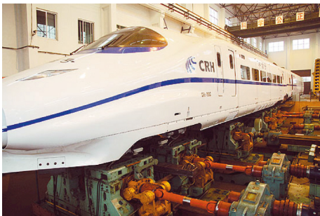
FIGURE 10: Actual rolling and vibration test rig of the vehicle in the key laboratory of rail transportation of Southwest Jiaotong University.
