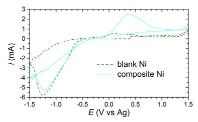
**Figure 3.** Cyclic voltammetry curves recorded in a blank Ni plating bath and suspension bath containing 2 g dm $^{-3}$  Ce<sub>2</sub>(MoO<sub>4</sub>)<sub>3</sub> 4.5H<sub>2</sub>O microflakes, at 70 °C on a rotating disk electrode with Pt tip (3 mm diameter), at 600 rpm.
