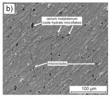
**Figure 1.** Surface morphology of (a) blank and (b) composite Ni coatings deposited on the copper substrate at a current density of 6 mA cm $^{-2}$  at 70 °C for 1 h, and (c) as-synthesized cerium molybdenum oxide hydrate microflakes for comparison. Pictures were recorded in a SE mode of SEM.
