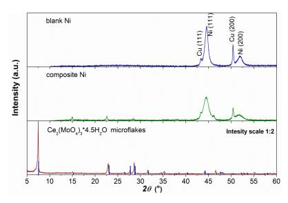
**Figure 2.** X-ray diffractograms for blank and composite Ni coatings deposited on the copper substrate at a current density of 6 mA cm $^{-2}$  at 70 °C for 1 h. A powder diffraction pattern for as-synthesized cerium molybdenum oxide hydrate is also shown at the bottom of the figure for comparison.
