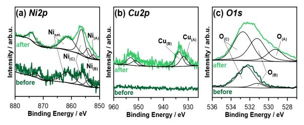
**Figure 9.** High-resolution XPS spectra recorded for blank Ni coating in (a) Ni2, (b) Cu2p, and (c) O1s peak binding energy range, before and after the exposure to 0.05 M NaCl.
