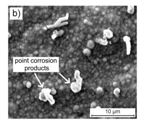
**Figure 11.** Surface morphology of (a) composite and (b) blank Ni coatings (deposited on the copper substrate at a current density of 6 mA cm $^{-2}$  at 70 °C for 1 h) after one-week exposure to 0.05 M NaCl solution.
