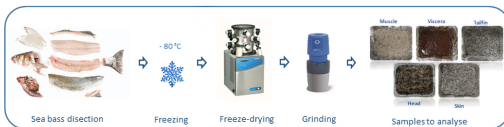
Figure 1. Scheme of sea bass side stream sample preparation.
