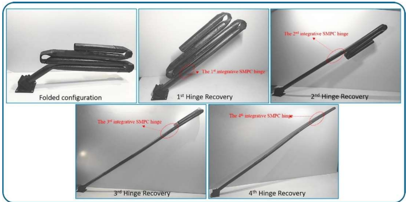
Figure 23. Shape memory recovery process of self-deployable structure. Reprinted/adapted with permission from Ref. [111].
