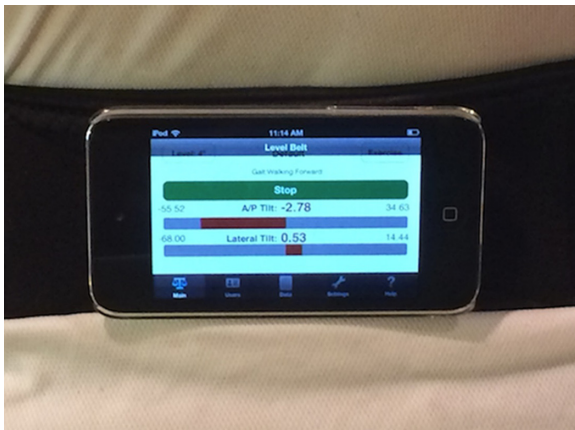
Figure 2 Placement and screen display of iPod Touch Level Belt measuring lumbopelvic tilt during a 40 m walk.
