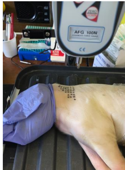
Figure 2. Piglet cadaver positioned with needle attachment directly above the neck injection site (dotted triangle).
