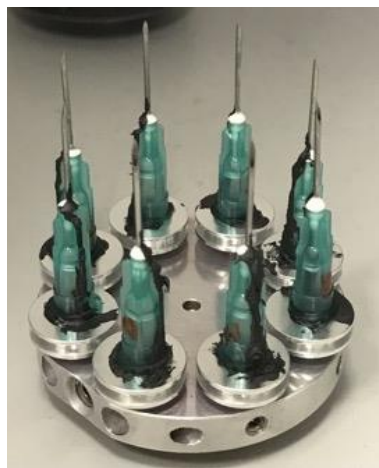
Figure 3. Needles mounted on aluminium specimen stubs with Leit-C to form a conducting strip from the base of the hub to the needle shaft.
