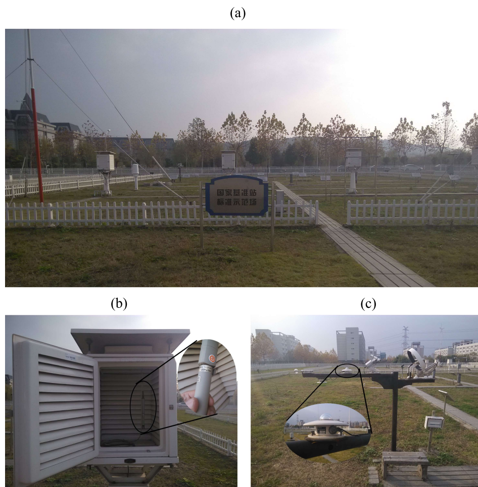
Figure 6. National weather station at NUIST, China, No. 59606. (a) Panorama of the AWS; (b) the meteorological temperature sensor (HMP45D) in the thermometer screen in the AWS; (c) the pyranometer (TBQ-2-B) in the AWS.
