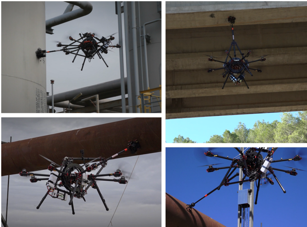
Figure 3. AeroX in contact inspection of surfaces with different positions orientations in different outdoor experiments and with different end-effectors: inspecting pipes ( bottom-left and bottom-right ), horizontal ceilings ( top-right ) and vertical surfaces ( top-left ).
