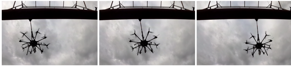
Figure 9. AeroX during contact flight in an experiment performed in Seville in October 2018. AeroX was flying in autonomous mode and the end-effector was teleoperated by the inspector. Images at different times show the motion of the end-effector along the pipe while keeping the relative position of the aerial vehicle.
