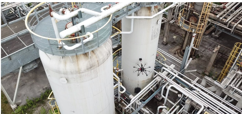
Figure 1. AeroX performing an ultrasonic thickness measurement in a refinery located in Germany in 18 July. The exact location cannot be disclosed due to confidentiality issues.
