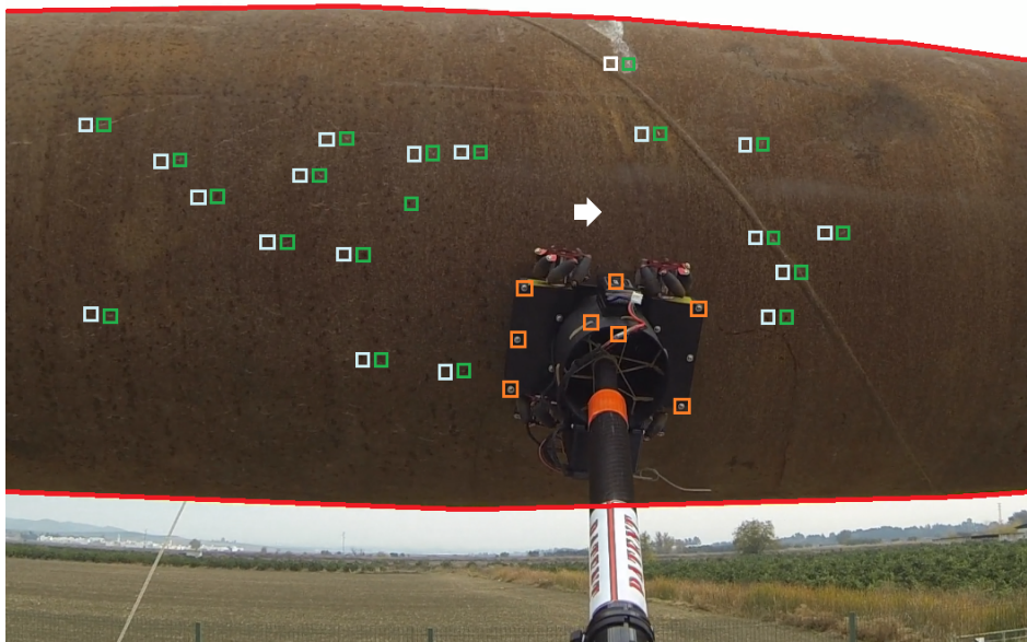
Figure 8. Picture of the on-board camera used for the visual-based relative localization system. The green rectangles are used to mark the SURF features in FS_t that were correctly matched—after executing RANSAC—with features in FS_{t-1} ,—marked with white rectangles. The matchings (of the end-effector) filtered out by RANSAC are marked with red rectangles. A small white arrow illustrates the relative displacement between the end-effector and the pipe between t - 1 and t .
