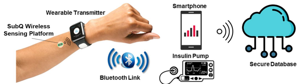
Figure 1. Components of the smart closed-loop diabetes management system 1. Subcutaneous wireless sensing platform 2. Wearable Transmitter 3. BLE Link from Transmitter to external reader 4. Smartphone and/or Insulin pump as external reader 4. Wireless Link to a secure Cloud 5. Secure Cloud.
