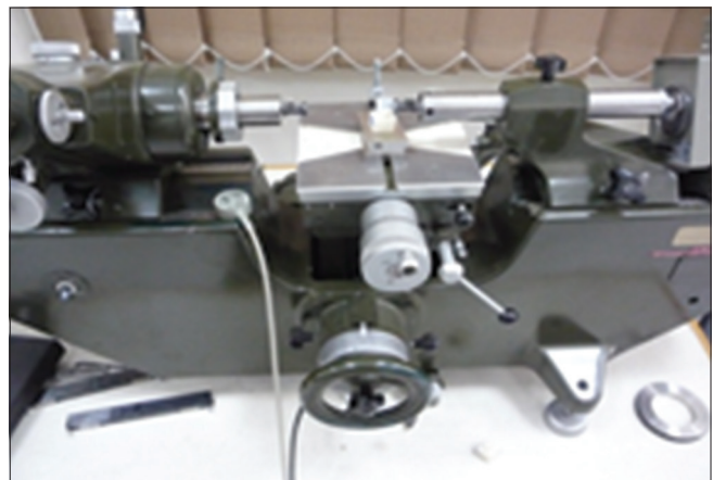
Figure 3: Universal horizontal metroscope
