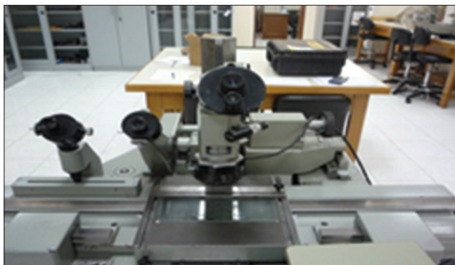
Figure 2: Universal measuring microscope
