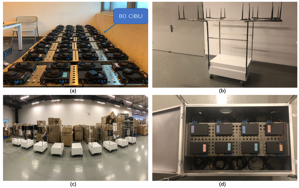
Figure 22. (a) 80 OBU for indoor testing, (b) background vehicle, (c) 8 background vehicles, (d) Box of the vehicle and 8 OBUs.
