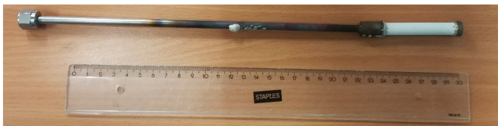
Figure 1. Picture of the sealed (by means of the reactive air brazing (RAB) sealing technique) MgO porous membrane used to carry out the membrane reactor experiments.
