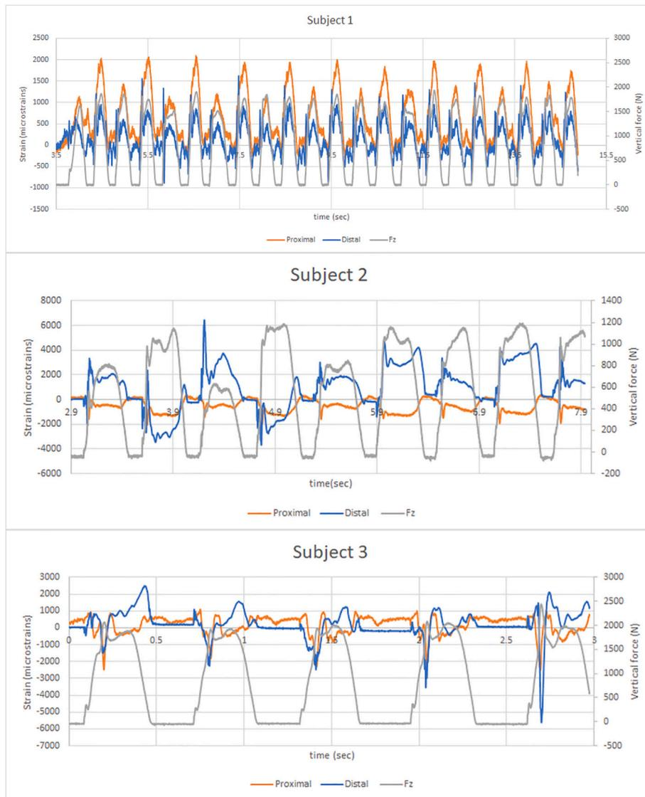
**Fig. 3.** Inter subject differences in proximal and distal tibial strains while performing serial vertical jumps on a force plate for three subjects. The interval between two vertical lines represents 0.5 s of time. Strain output from the proximal gauge is presented in green, from the distal gauge in blue and from the force plate in grey.
