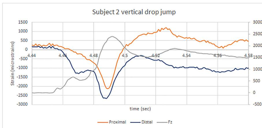
**Fig. 4.** The differences in proximal and distal tibial strains while Subject 2 performed a vertical drop jump on a force plate. The interval between two vertical lines represents 1 s of time. Strain output from the proximal gauge is presented in green, from the distal gauge in blue and from the force plate in grey.
