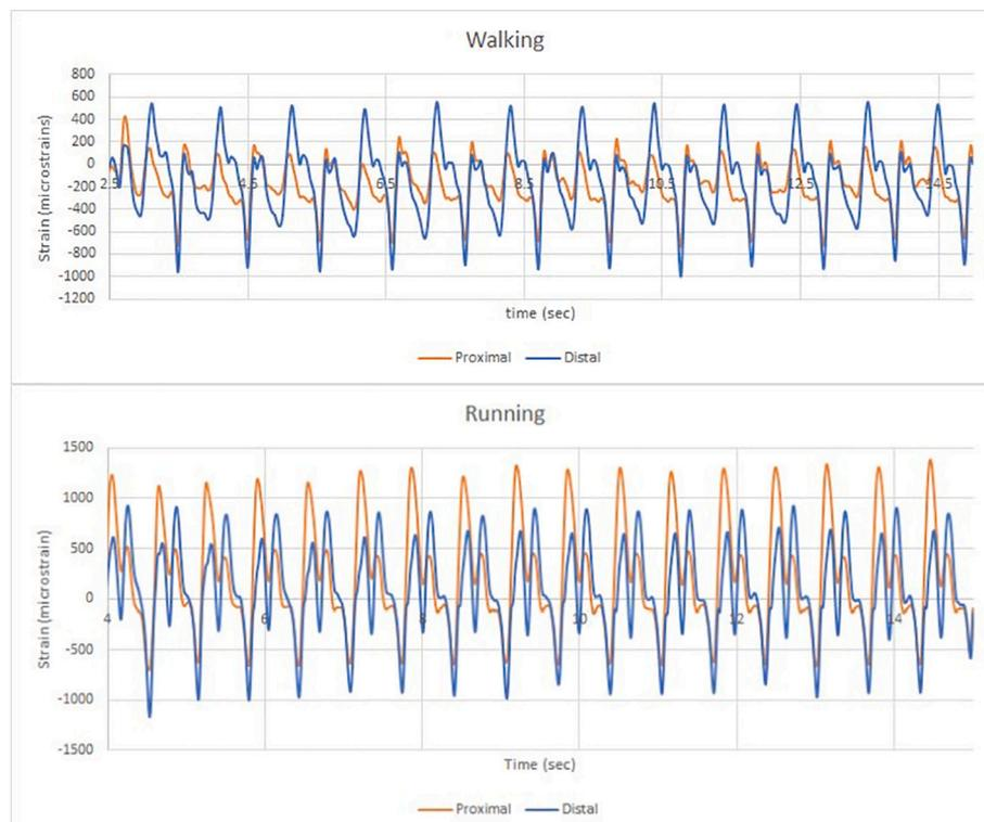
Fig. 2. Proximal and distal tibial strains during treadmill walking and running for Subject 1. The interval between two vertical lines represented 2 s of time.
