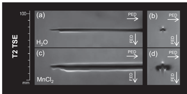
FIGURE 5 Artifact diameter of MRI compatible microwave therapeutic antennas can be enhanced by filling the cooling circulation system with fluid contrast agent instead of water. Angulation to B_0 was 90^\circ , (a) and (c) show coronal, (b) and (d) show axial slice orientation for the example of the T2 TSE sequence. The cooling circulation system was either filled with water (a, b) or 5 mmol/ml MnCl_2 (c, d).
