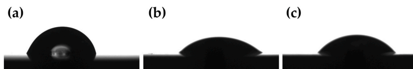
Fig. 7. Representative images of contact angle measurement on etched lithium disilicate ceramic discs, as measured for high purity water (a); SBU (b) and SBP (c).
