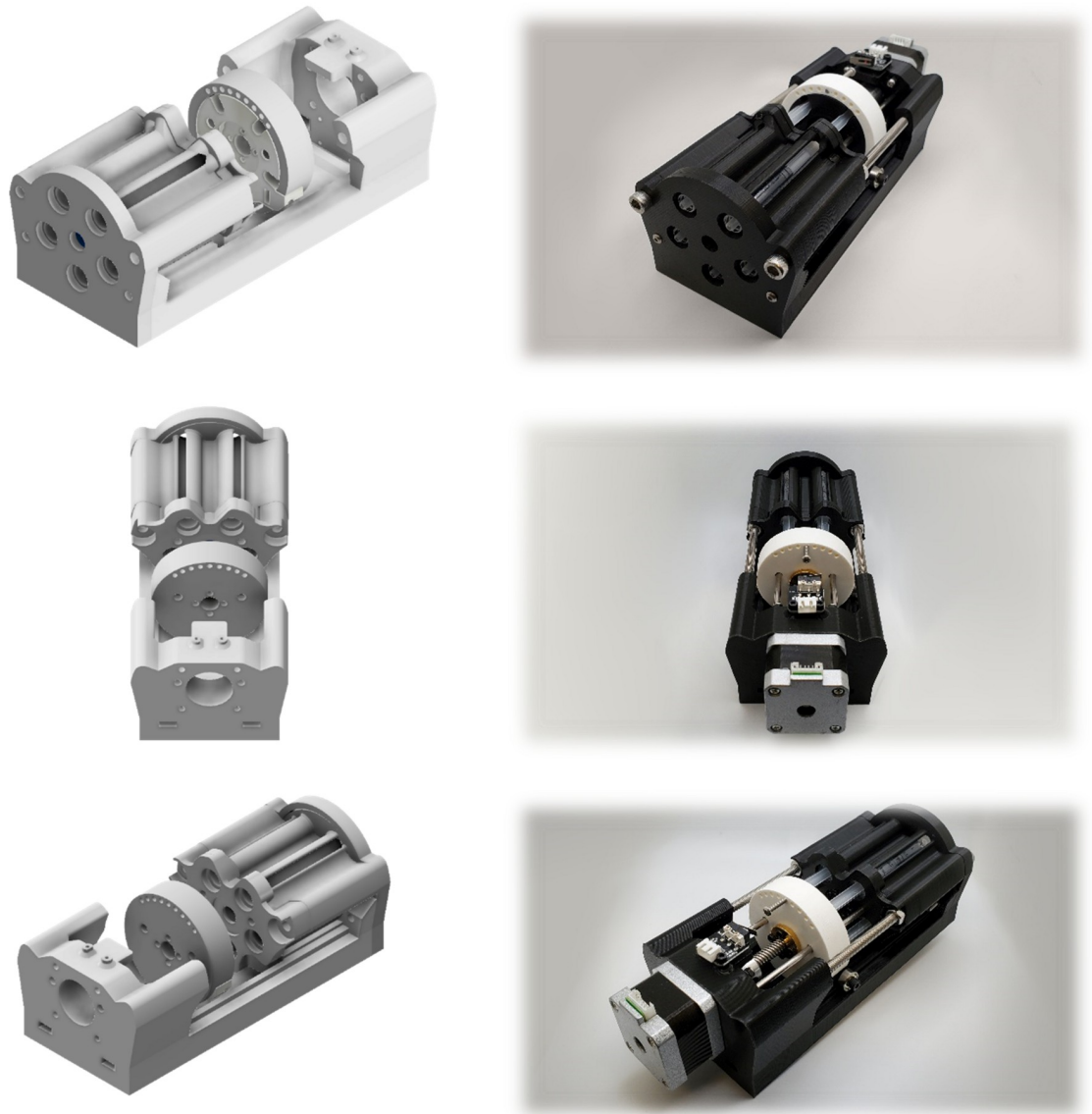
Fig 1. Reciprocating positive displacement pump. Syringe pump unit CAD models ( left ). A fully assembled unit with 3D printed parts and other components ( right ).
