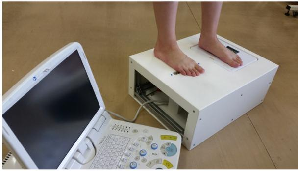
**Fig. 1.** Weight-bearing plantar ultrasound-imaging device. One forefoot (right foot in this case) was placed on a solid gel block for ultrasound evaluation and the other foot was placed on a digital weighing scale. The scale is used to measure the body weight on the foot to measure on the opposite side.
