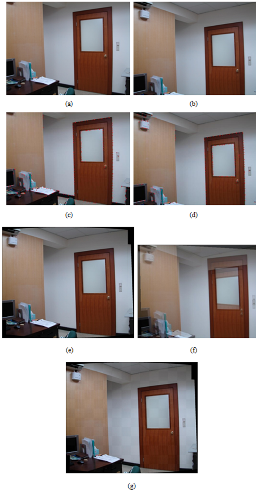
Figure 3. Registration result of indoor desk and door. (a), (b) An image pair used for registration, (c), (d) results of feature point extraction from (a) and (b), respectively, (e) registered result with proposed algorithm, (f) registered result by optical flow-based approach, (g) checkerboard visualization after the registration by proposed algorithm. doi:10.1371/journal.pone.0066656.g003
