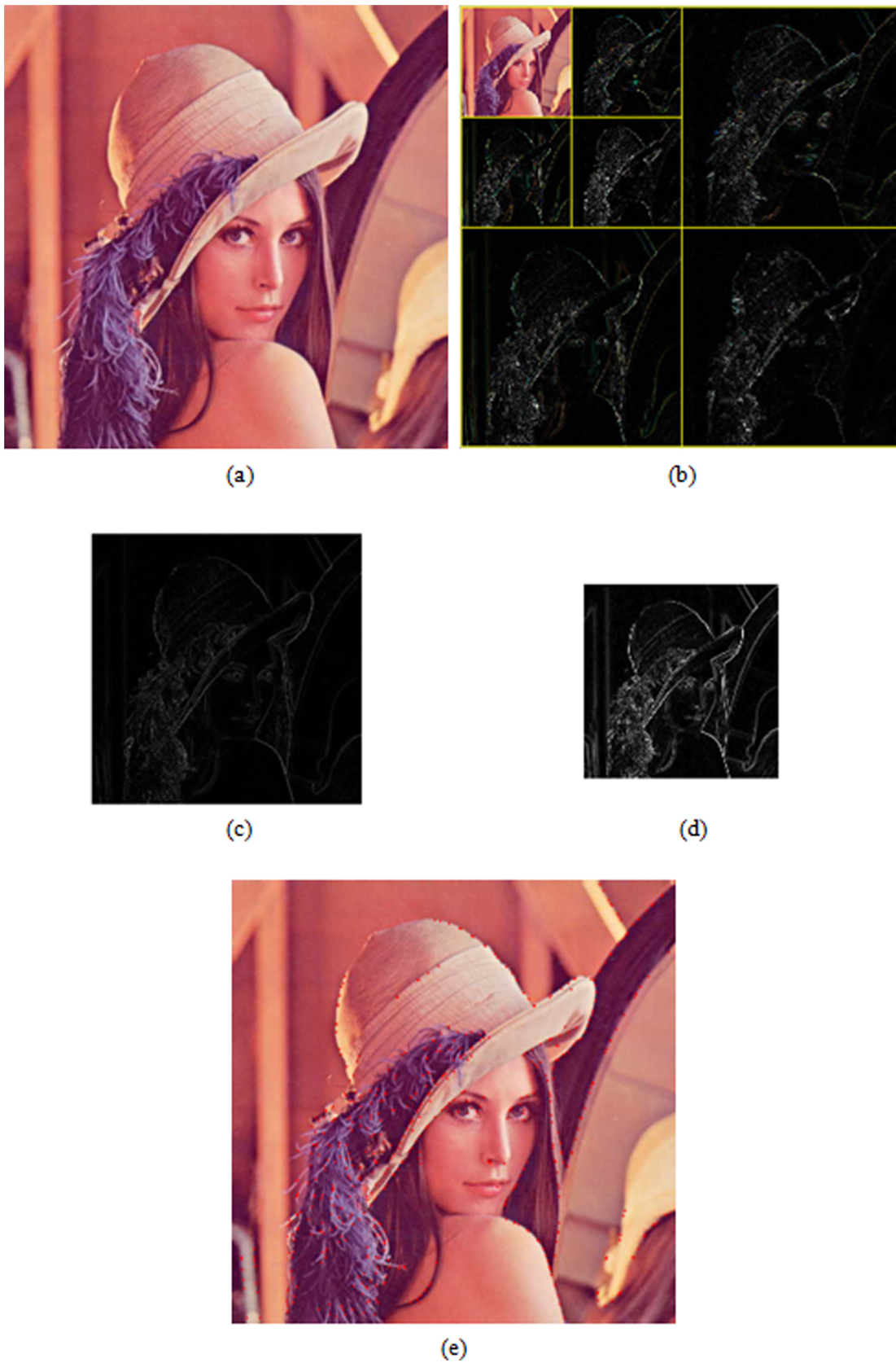
Figure 2. Procedure of feature extraction. (a) A test image, (b) 2D 2-level wavelet decomposition of test image (c), (d) gradient moduli (calculated from LH and HL quadrants) at level 1 and 2, respectively, (e) result of feature point extraction. doi:10.1371/journal.pone.0066656.g002
