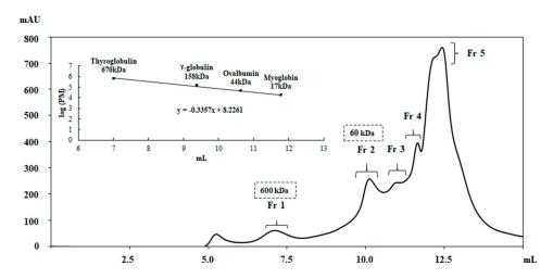
**Figure 7.** Elution profile of pellet 50% sample obtained by gel filtration chromatography performed on YARRA™ SEC-4000 column in 50 mM sodium acetate buffer pH 5.0 containing 50 mM NaCl. Insert: Calibration curve of the gel filtration YARRA™ SEC-4000 column using protein standards of known molecular masses. The collected fractions are indicated.
