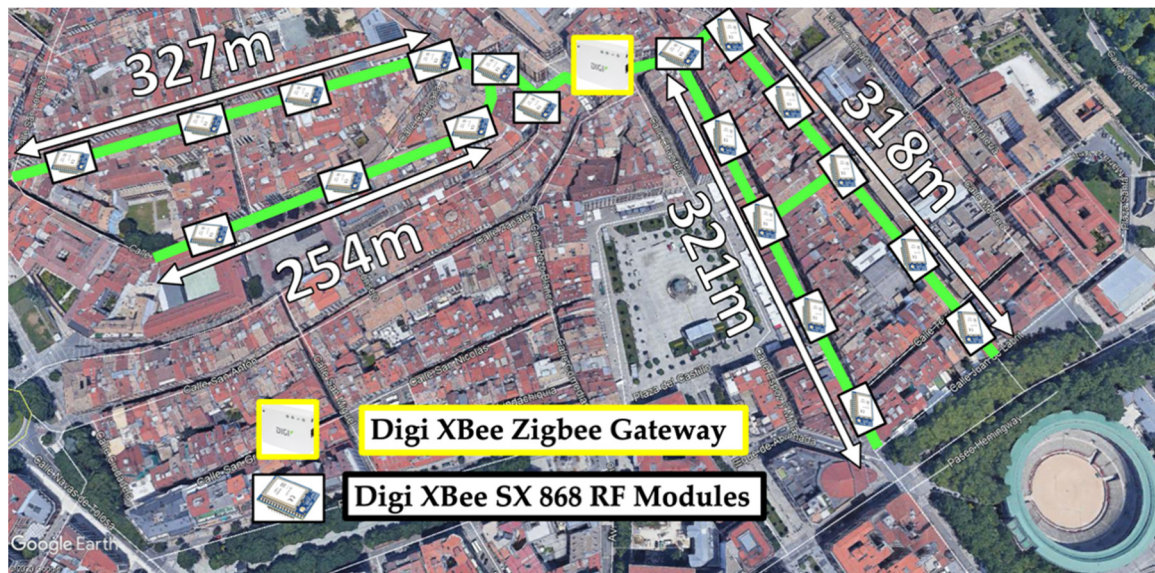
Figure 17. Schematic view of the proposed ZigBee 868-MHz WSN deployment.
