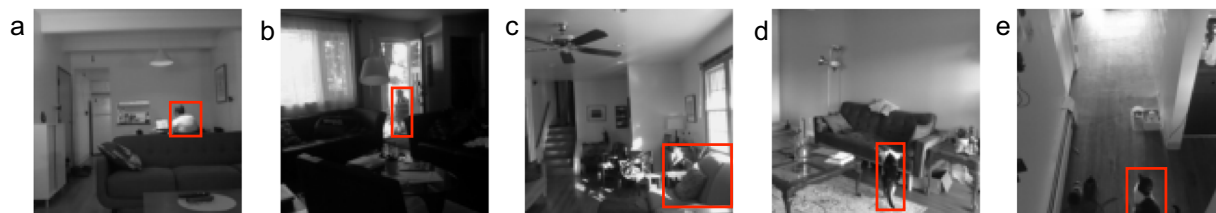
Fig. 7 Five images that were misclassified by the YOLOv5 labeling algorithm. (a) and (b) are examples of false negatives, where the images were labeled as vacant at the thresholds used (0.3 and 0.4, respectively). (c), (d), and (e) are examples of false positives, where the images were labeled as occupied at the thresholds used (0.5, 0.3, and 0.6, respectively). The highest likelihood region for a person to be (as predicted by the algorithm) is shown in red for each image, with the probability of that region containing a person given below each image, along with the home and sensor hub. (d) and (e) both highlight cats as the most probable person location, which occurred infrequently.
