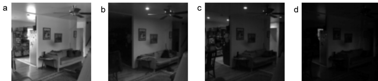
Fig. 3 Four different images from the same sensor hub, comparing the relative “brightness” of the images, as described by the average pixel value. The images shown are 112 \times 112 pixels. (a) Average pixel brightness: 106. (b) Average pixel brightness: 43. (c) Average pixel brightness: 32. (d) Average pixel brightness: 10.
