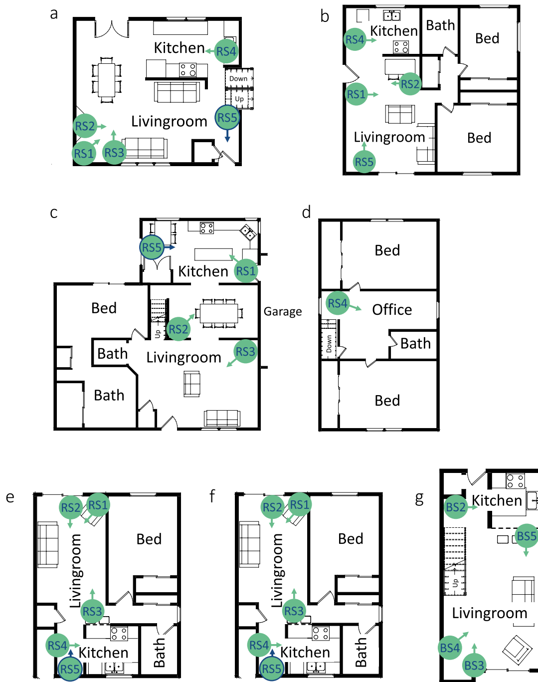
Fig. 2 Home layouts and sensor placements. Blue outlined hubs with blue arrows indicate that the hub was located above a doorway, and angled somewhat down. (a) H1: Main level of three-level home. (b) H2: Full apartment layout. (c) and (d) H3: Main and top level (respectively) of three-level home. (e) H4: Main level of two-level apartment. (f) H5: Full apartment layout. (g) H6: Main level of studio apartment with lofted bedroom.
